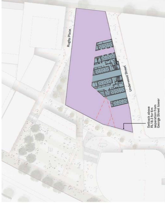
Figure_5.19. Reference design plan at typical podium level (up to ~20m (RL 24))
